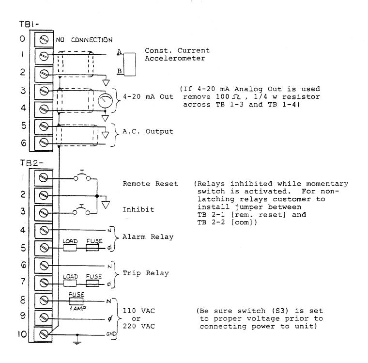
FIGURE 3 438D VIBRATION MONITOR CUSTOMER WIRING: FOR 4073 INPUT TRANSDUCER
