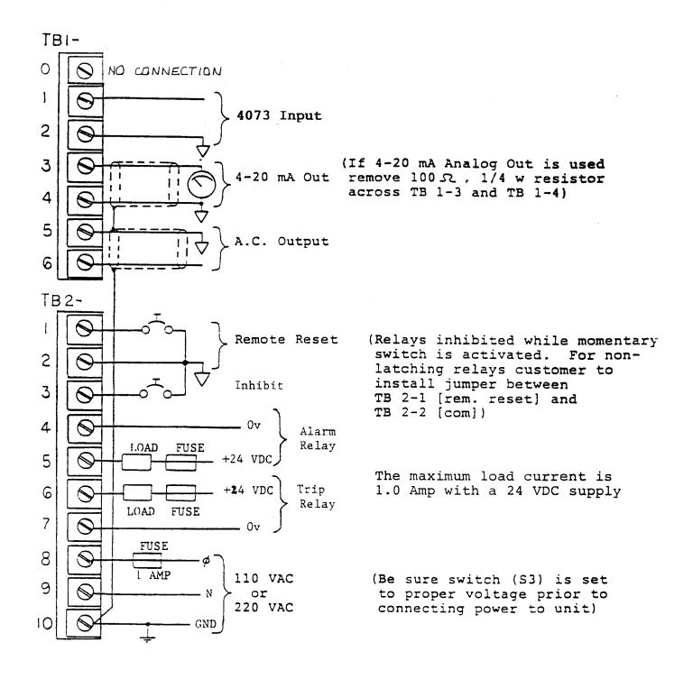
FIGURE 7 438D VIBRATION MONITOR CUSTOMER WIRING: FOR 4073 INPUT TRANSDUCER, AND SPECIAL 24VDC RELAYS
