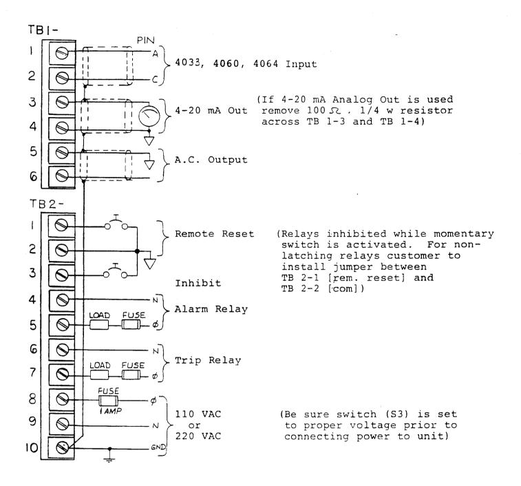
FIGURE 4 438D VIBRATION MONITOR CUSTOMER WIRING: FOR 4033 INPUT TRANSDUCER
