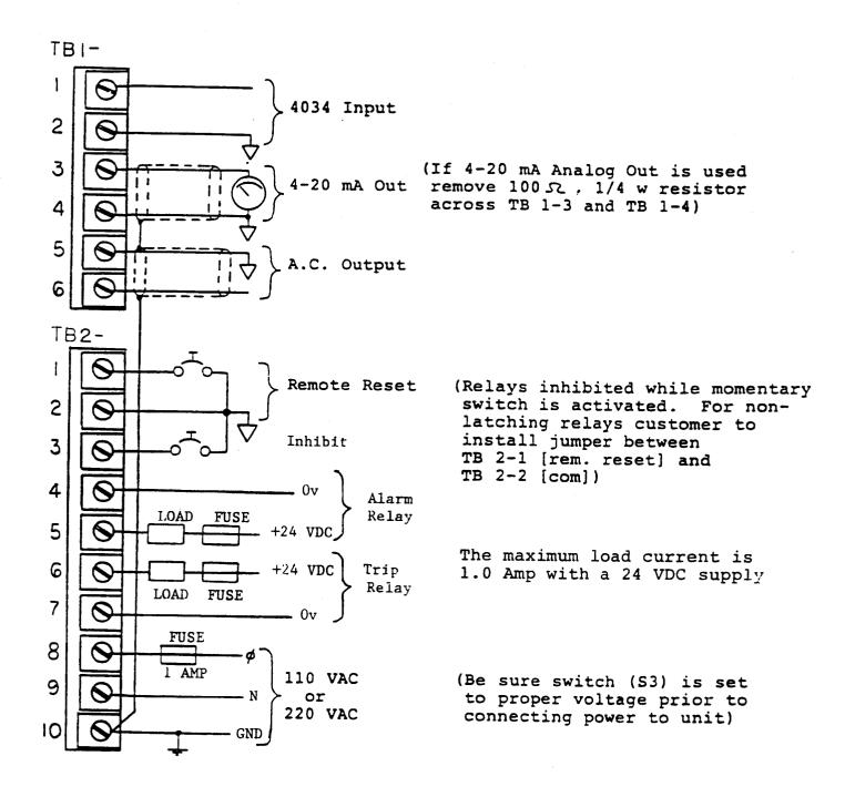
FIGURE 6 438D VIBRATION MONITOR CUSTOMER WIRING: FOR 4034 INPUT TRANSDUCER, AND SPECIAL 24VDC RELAYS
