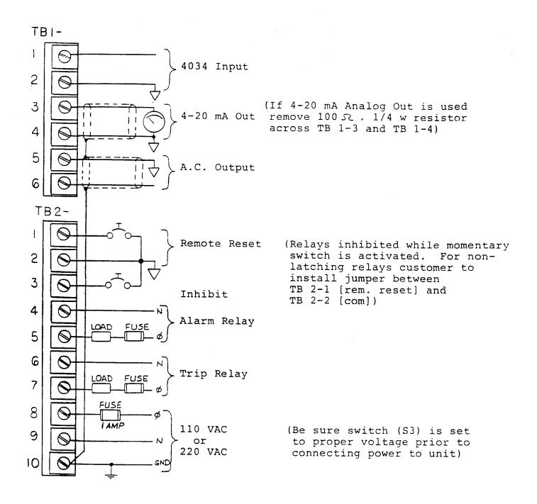
FIGURE 2 438D VIBRATION MONITOR CUSTOMER WIRING: FOR 4034 INPUT TRANSDUCER
