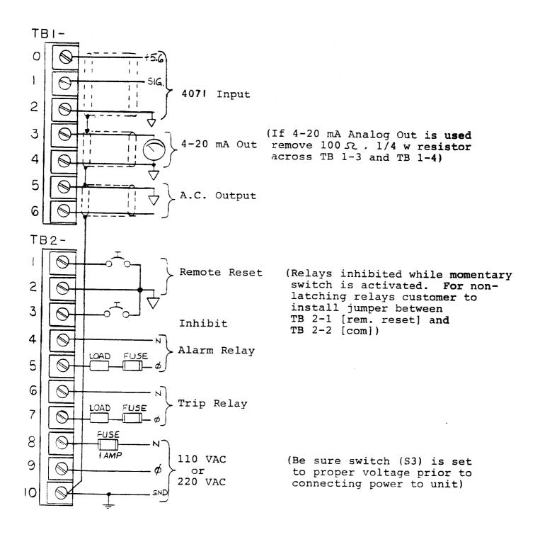
FIGURE 5 438D VIBRATION MONITOR CUSTOMER WIRING: FOR 4071 INPUT TRANSDUCER
