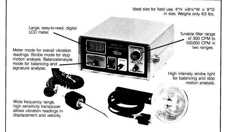
The Vitec **Model 655 Compact Balance Analyzer** is used for in-place balancing, vibration measurement and stop-motion analysis of rotating machinery.
